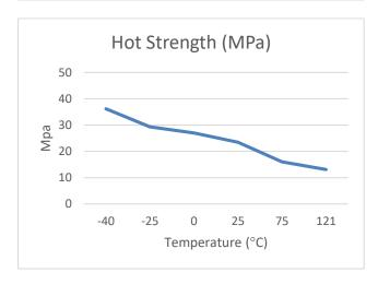
Lap Shear Strength ASTM D 1002 304 Steel / 304 Steel
